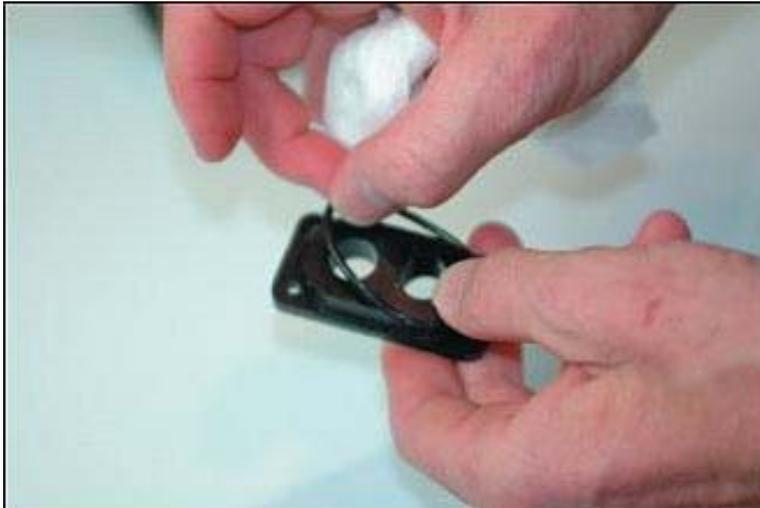
14. Press the bracket into position around the syringe barrels. Note that if the syringe sizes have been changed, a different sized bracket will be required for the new syringes.
