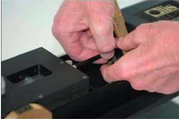
3. With the Fill/Flow valves in the Fill position, pull back on the plungers of drive syringes until they are removed from the stopped flow.
