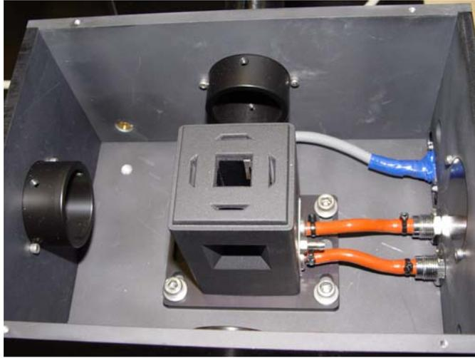
3. Locate the stopped flow assembly. Grasping the main assembly with your left hand and the ball of the drive plunger with your right hand. Note the stopped flow may or may not have legs attached to the right side (under the drive plunger). If no legs are present locate these prior to moving the stopped flow.
