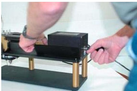
2. Lift the plunger block up and secure it to the shaft with a rubber band to keep the block out of the way.
