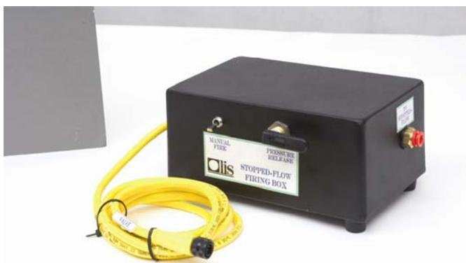
7. Connect the black gas tubing from the apparatus to the stopped flow firing box. Push the tubing into the port labeled 'to SF'. Pull gently to assure a proper connection.
