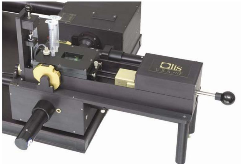
4. Lift the assembly into the sample chamber so that it fits snugly into the chamber. Gently wiggle the stopped flow to assure it is securely in place. Fasten the stopped flow to the chamber using four 3/32" Allen screws. If the stopped flow legs were not present on the apparatus, attach these now by sliding the legs under the right side of the stopped
