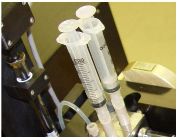
3. Replace the reservoir syringes with syringes containing the desired solvent or buffer.
