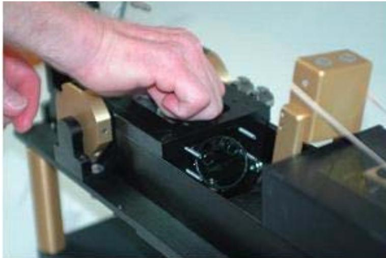
11. Insert the stopped flow tool into the base of the syringe and rotate the syringe counter-clockwise. Carefully remove the syringe by sliding it out the right side of the bath. Repeat for the second syringe.
