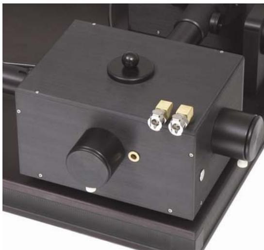
2. If a Peltier cell or turret is present, this must be removed prior to installation of the stopped flow. If no cell holder is present, proceed to the next step. Remove the screws holding this to the base plate. Remove the 3/32" four screws holding the side panel on the sample chamber. Place the whole assembly aside. Obtain the sample chamber side panel to be used with the stopped flow.
