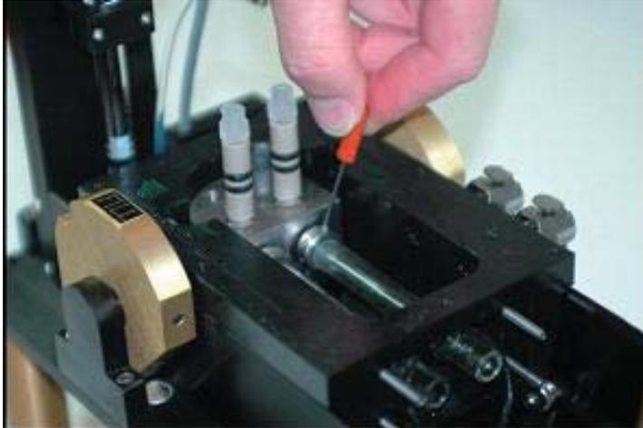
12. Insert the new syringes into the bath. Screw them clockwise into the valve using the stopped flow tool. Tighten the syringes until they are snug. Exercise care not to over tighten the syringes. This may cause them to leak.
