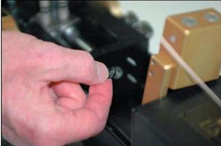
16. Replace the outer half of the syringe plunger bracket and replace the thumb nuts and purge fitting.
