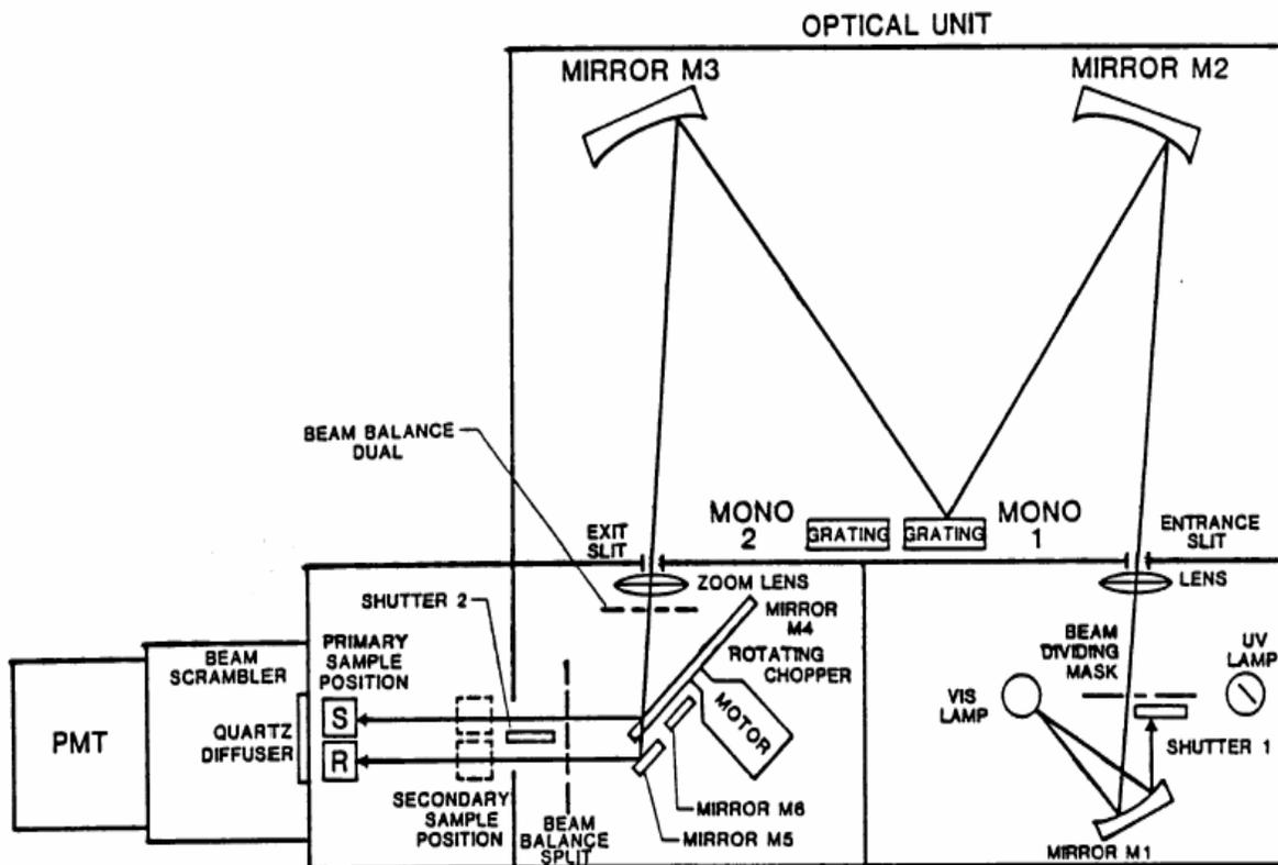
Aminco DW-2000 double-beam mode functional diagram
