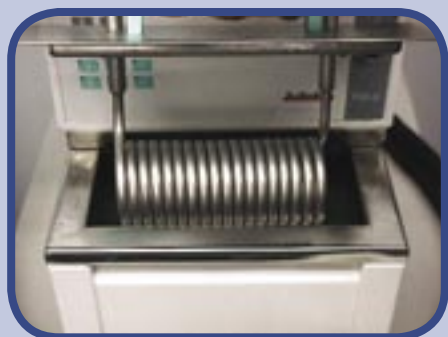
Olis-added circulating coil to preferred water bath.
