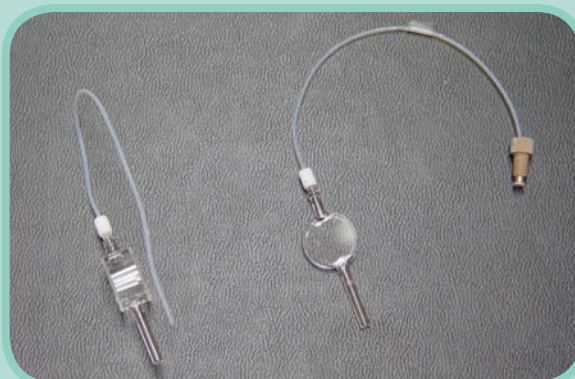
Long and short pathlength flow-thru cuvettes
